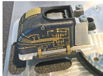
Yamaha SMD mounting equipment for 3D-MIDs also uses a 3D-MID
